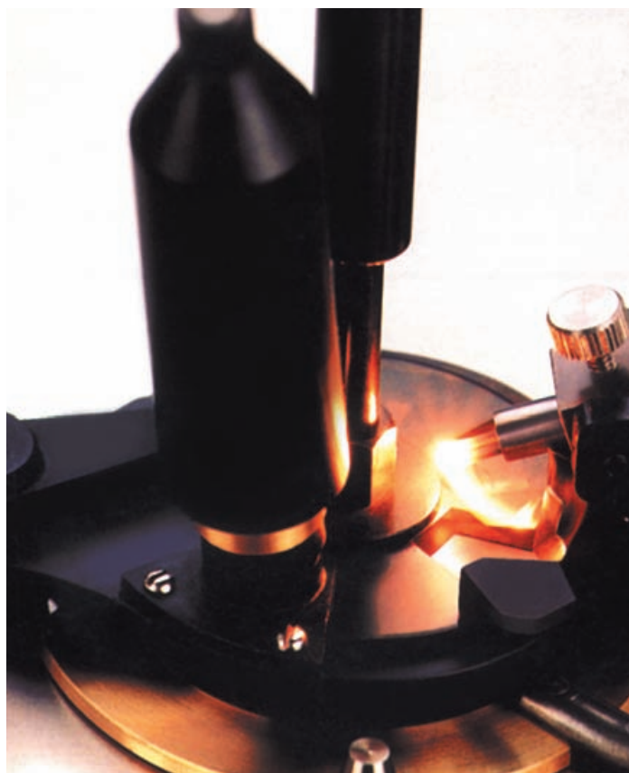
Automated Tag closed Cup Flash Point Tester
