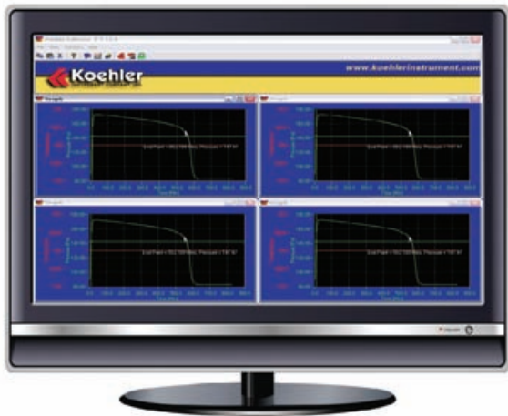
Real-time plot screens display pressure versus time for up to twelve samples simultaneously (four different test methods shown).
