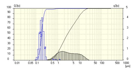
1-43 quartz sand 30 min PULVERISETTE 6, dry grinding, 250 ml  $ZrO_2$  bowl, 20 mm balls, average quartz sand 120 min PULVERISETTE 6, wet grinding, 2nd step, 250 ml  $ZrO_2$  bowl, 320 g of 0.4 mm  $ZrO_2$  balls 3rd test series, average
